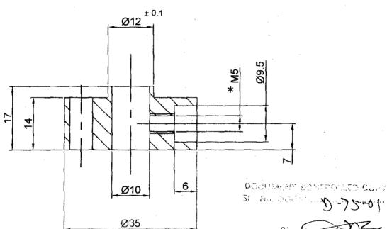
MATERIAL - MS FINISH - ZINC YELLOW QTY. - 01 / MC. NOTE: -DRG NO. ITI/TR/012 TO BE PRESS FITTED IN HOLE Ø6 H7 SUPPLY MUST BE IN ASSY.
