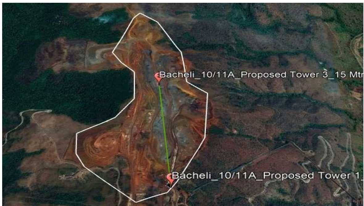
Fig 36 Bacheli 10/11A Wireless Link for AP#3
