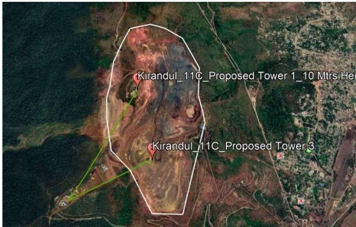
Fig 18 Kirandul 11C Wireless Link
