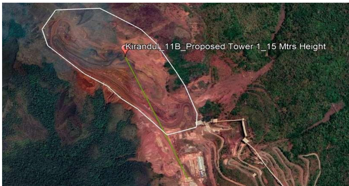
Fig 14 Kirandul 11B Wireless PTP Backhaul
