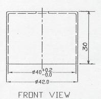
ote : Ø5.0mm hole provided on center of the top surface is acceptable.
